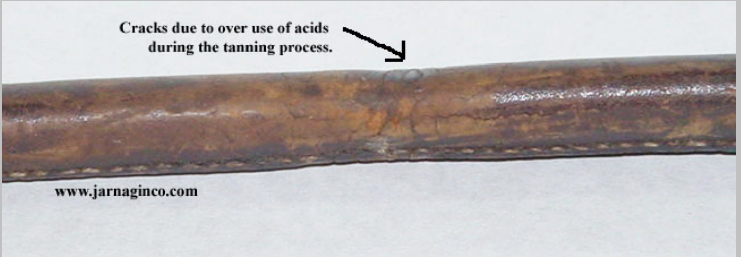
Figures 2A & B. Hemlock tanned 1859 pattern two rivet bayonet scabbard. Note acid damage in bottom photo.
