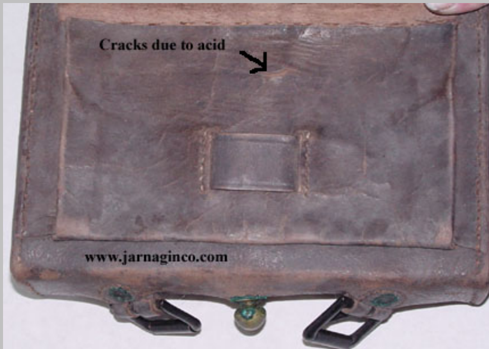
Figure 3: Hemlock tanned Watertown Arsenal cartridge box. Note cracks in leather due to acid
